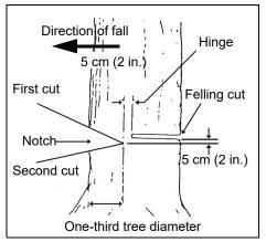
direction. When the tree starts to fall, kill the engine, place the saw on the ground and make your retreat quickly.
