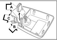
Note: For operation at normal temperature 5° C (41°F) return the plug to its original position. To prevent over-heating of the engine.
