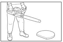
Move chain brake lever fully REARWARD to UNLOCK chain brake.
