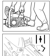
Note: Do not pull starter rope out to the maximum possible position. Do not allow recoil handle to snap back against the case. If engine does not start after five pulls, repeat instructions. Do not increase engine speed while chain brake is locked. Severe brake damage will result.
