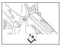
7. Be sure that saw chain stops moving when throttle trigger is released.
