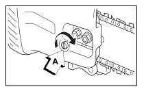
4. Tighten nuts with the bar nose held up.
