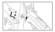
4. Securely hold the chainsaw as shown and pull starter handle.
