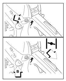
Securely hold the chainsaw 7. and pull starter handle several times until first starting sound.
