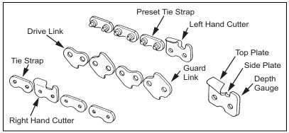
Important points for proper maintenance of saw chain:
