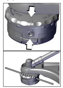
Hold trimmer head while turning knob clockwise to wind line onto spool until about 13 cm (5 in.) of each line remains exposed.
