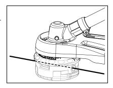
Hold trimmer head while turning knob clockwise to wind line onto spool until about 13 cm (5 in.) of each line remains exposed.
