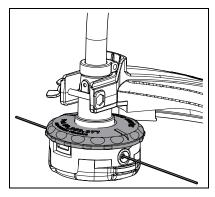
Hold trimmer head while turning knob clockwise to wind line onto spool until about 13 cm (5 in.) of each line remains exposed.
