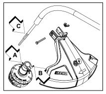
5. Install the bearing housing and shield.
