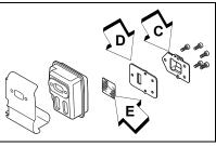
Use a wood or plastic scraping tool to clean deposits from cylinder exhaust port (C).
