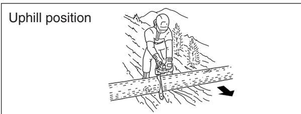
Keep in mind that the wood is heavy and that it will bend and pinch the saw if improperly supported.
