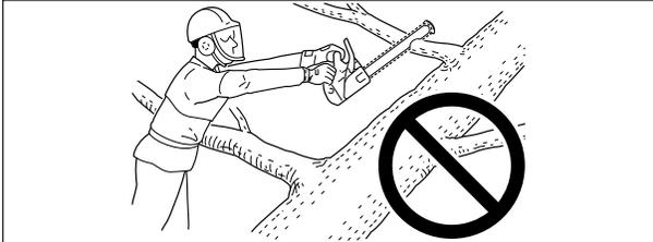
Don't cut with the saw overhead or aligned vertically with your body.
