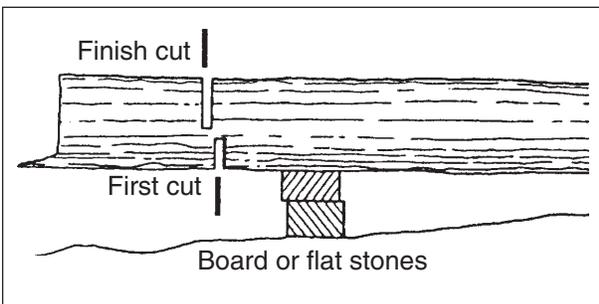
To cut the trunk, use the bucking and two-cut sequence shown.
