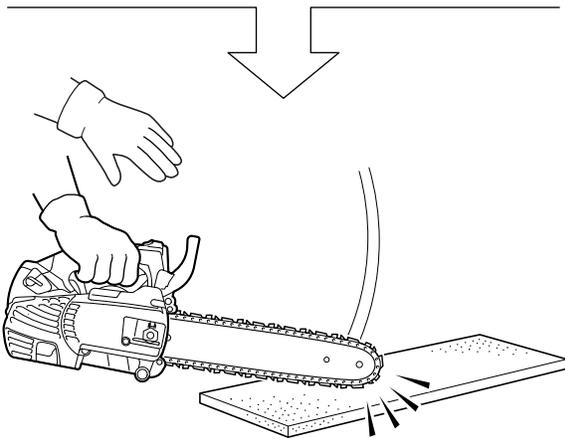
Rear handle should be gripped lightly with the right hand.
