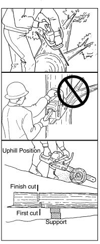
Keep in mind that the wood is heavy and that it will bend and pinch the saw if improperly supported. The trunk will weaken at the point where you make the cut unless the tree is lying on perfectly flat ground or supported as shown. If you make the cut with the tree on the ground, don't let the saw's chain dig into the earth; it is harmful for the saw, and you stand a good chance of being struck by flying debris.
