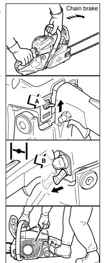
8. Push choke control knob all the way IN (OPEN [] ∤ ]]choke position).
