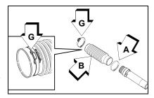
Assemble flexible pipe to elbow (D) on blower. Position clamp with cable guide loop (G) on outside of flexible pipe and tighten clamp.
