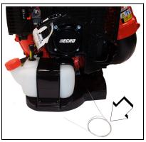
2. Route the anti-static wire below the fan housing and clip the wire into throttle cable retaining clip (X). Position the wire outside of the blower elbow.
