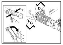
Position throttle cable along the outside of elbow. Loosen knob (H) on handle (E). Align notches in handle with tabs (F) and install onto swivel pipe (C) past long ridges in pipe.
