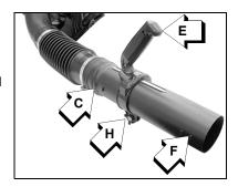
Assemble straight pipe (J) onto swivel pipe (C), until you feel light resistance. Do not force connection. Hold swivel pipe and turn straight pipe clockwise, engaging positive locking channels, until connection is firm. Do not force connection.
