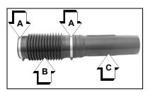
Assemble flexible pipe (B) to elbow (D) on blower and tighten clamp (A).
