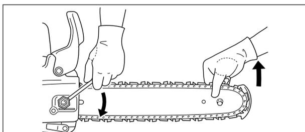
4. Mount guide bar on stud and slide toward clutch to make saw chain installation easier. Install chain with cutters on top of guide bar facing forward.
