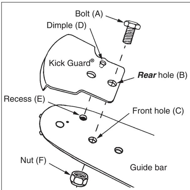
1. Install bolt (A) in **rear** hole (B) of Kick Guard® and through front hole (C) in guide bar.
