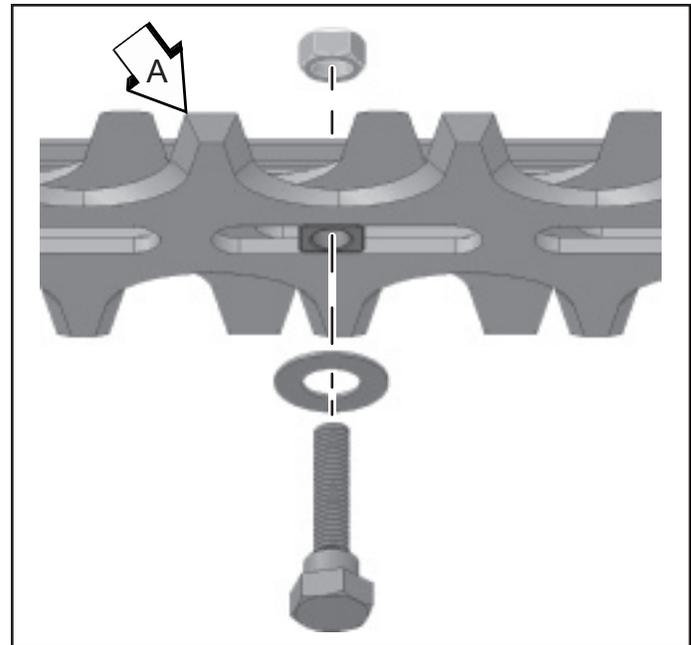
3. Hold the lock nut and loosen the bottom spacer bolt 1/2 turn counterclockwise to allow for blade clearance. Keep blade gaps a minimum of 0.127 - 0.20 mm (0.005 - 0.08 in.) for best cutting performance.
