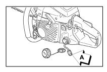
Pull filter out through gas port, and inspect filter.
