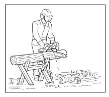
Sap from palm trees may corrode metal parts unless proper saw maintenance is performed. Make sure to clean metal parts from palm sap immediately after use.
