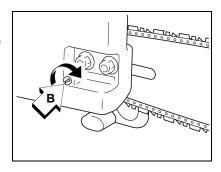
4. Tighten nuts with the bar nose held up.
