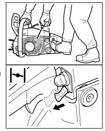
5. Choke may be used if necessary, but after first starting sound, squeeze throttle trigger to release choke and return engine to idle.
