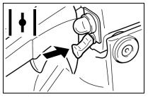
Do not allow recoil handle to snap back against the case.
