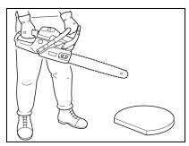
2. Move chain brake lever fully REARWARD to UNLOCK chain brake.
