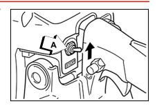
Securely hold the chain saw as 4. shown and pull starter handle.
