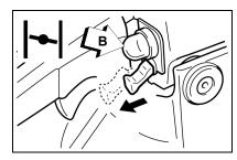
Securely hold the chain saw 7. and pull starter handle several times until first starting sound.
