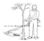
To free a blade that is bound in the cut, stop the engine, and support the trimmer or brushcutter to
