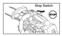
authorized dealer to check and repair Stop switch before starting the engine again.
