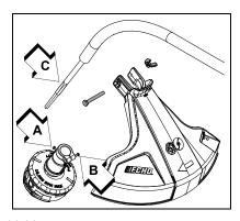
5. Install the bearing housing and shield.
