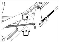
Insert other end of lower control rod into hole in gate control (H), as shown, and secure with clevis pin (I).
