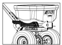
Pull gate control lever backward to set gate to desired opening size. Use gate adjustment limiter (B) to restrict gate opening size.
