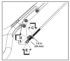
3. Insert lower control rod (F) into hinge (G), as shown.
