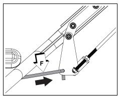
6. Position gate control lever fully forward, and tighten upper control rod nut and flange nut as shown.
