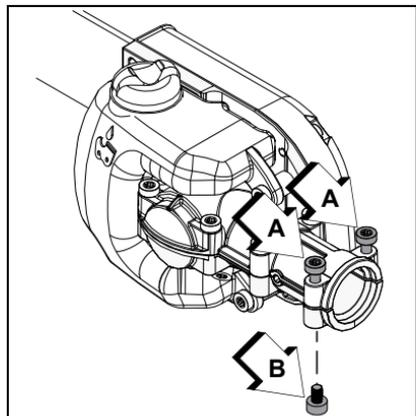
3. Slide the cutting attachment onto the shaft housing until the hole in the neck of the cutting attachment is aligned with the hole (C) in the housing (it may be necessary to rotate the saw chain slightly to align the internal pinion and drive shaft).
