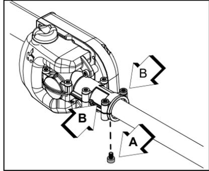
4. Remove flex cable (C), wipe clean and apply 15 ml (0.5 oz.) of lithium based grease.
