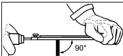
5. Place depth gauge tool firmly on top of cutter with 0.635 mm (0.025 in.) slot and end against front cutter raker. File cutter raker with flat file until flush with top of depth gauge.
