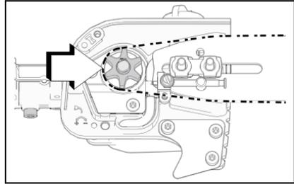
4. Hold the bar nose up. Install guide bar cover (D). Install the guide bar nuts (A). Tighten the rear nut first, then tighten the front nut. Install and tighten the guide bar cover screw (B)
