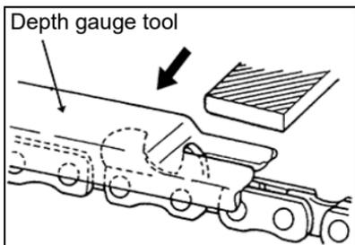
6. Finish cutter sharpening by rounding front raker edge with flat file.
