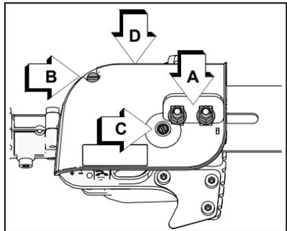
3. Gently brush debris from inside guide bar cover and from around sprocket.
