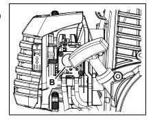
Lay the unit on a flat area and keep movable attachment parts clear of all obstacles. Firmly grip throttle handle and throttle trigger lockout with left hand. Rapidly pull recoil starter handle/rope (D) until engine starts.
