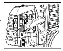
4. Lay the unit on a flat area and keep movable attachment parts clear of all obstacles. Firmly grasp throttle handle and throttle trigger lockout with left hand and fully depress throttle trigger to wide open position. Rapidly pull recoil starter handle/rope (D) until engine starts (or maximum five pulls).
