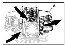
Dust and grass build up on the outside of the cylinder. This build up insulates the engine and prevents the heat from leaving.
