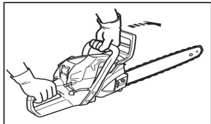
3. Securely hold the chainsaw as shown and pull starter handle.
