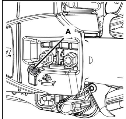
4. Tighten nuts with the bar nose held up.
