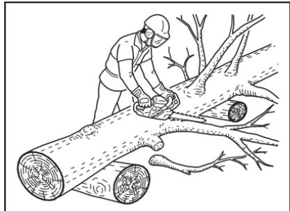
Do not cut with the saw overhead or aligned vertically with your body. If the saw should kick back, you may not have enough control to prevent possible injury.
