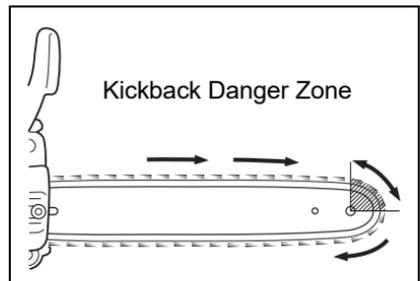
2. Keep a good firm grip on the saw with both hands, the right hand on the rear handle, and the left hand on the front handle, when the engine is running. Use a firm grip with thumbs and fingers encircling the chainsaw handles. A firm grip will help you reduce kickback and maintain control of the saw. Do not let go.
