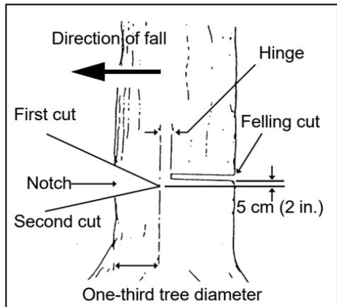
To fell big trees with a diameter exceeding twice the bar length, start the notching cuts from one side and draw the saw through to the other side of the notch. Start the back cut on one side of the tree, pivoting the saw through to form the desired hinge on that side. Then remove the saw for the second cut. Insert the saw in the first cut, very carefully so as not to cause kickback. The final cut is made by drawing the saw forward in the cut to reach the hinge.
