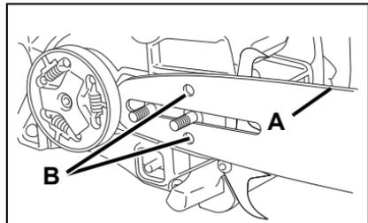
5. Clean the guide bar mount area before installing the guide bar.
