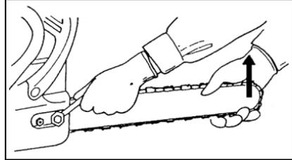
5. Pull the chain around the bar by hand. Loosen the adjustment if you feel tight spots.
