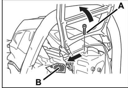
Note: When cleaning carbon deposit, be careful, do not damage the catalytic element inside muffler.
