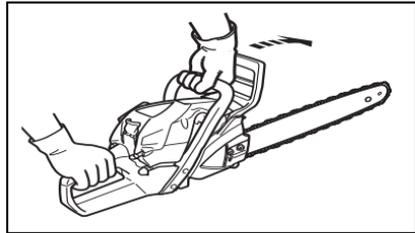
2. Press throttle trigger lockout (D) down while engaging throttle trigger (C).
