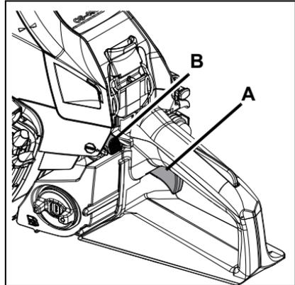
**Checking Chain Tension**
