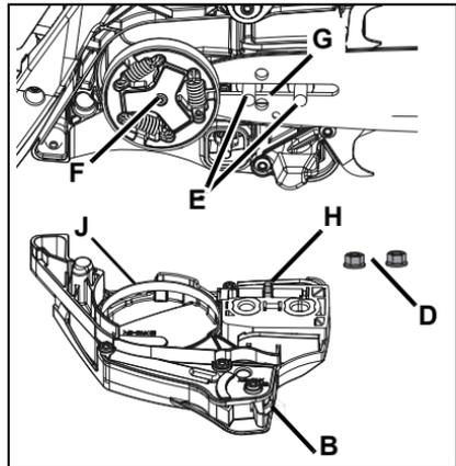
7. Turn saw over, and check brake band (J) for correct position on clutch drum. If brake band is not in place around drum, remove sprocket guard, and reinstall. Tighten sprocket guard nuts finger tight.
