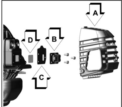
Note: When cleaning carbon deposit, be careful not to damage the catalytic element inside muffler.
