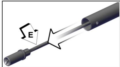
7. Slide coupler on upper drive shaft until fully seated, and align set screw hole in coupling with hole in upper drive shaft.
