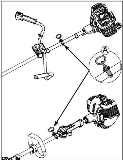
3. Slide harness clamp up (A) or down until unit balances with head or blade 200 mm  $\pm$  100 mm (8 in  $\pm$  4 in) from the ground (B).
