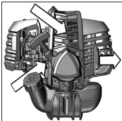
Removal of cooling passage blockages or cleaning of cooling fins is considered "Normal Maintenance". Any failure attributed to lack of maintenance is not covered by the warranty.
