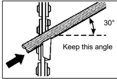
3. Keep file horizontal in cutter and file in one direction.
