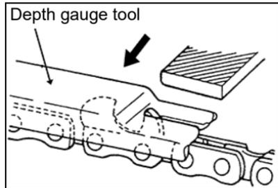
6. Finish cutter sharpening by rounding front raker edge with flat file.
