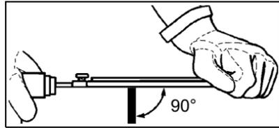
5. Place depth gauge tool firmly on top of cutter with 0.635 mm (0.025 in.) slot and end against front cutter raker. File cutter raker with flat file until flush with top of depth gauge.
