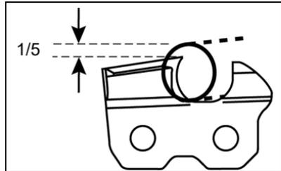
4. File until cutter top and side bevel edges are sharp without nicks.
