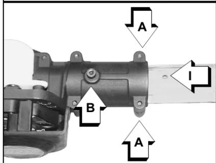
6. Install and tighten locator screw (B). Tighten two (2) cutting attachment screws (A).
