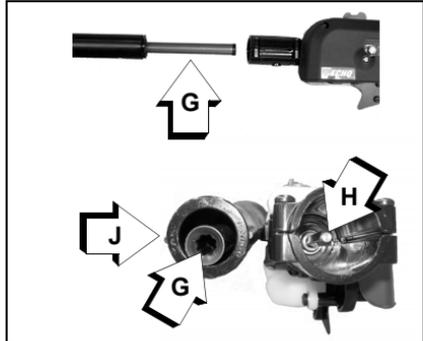
5. Slide together, aligning locator hole in cutting attachment with locating hole in upper tube (I).
