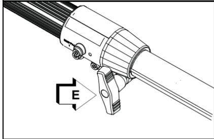
3. Pull upper tube (F) out of fiberglass lower tube 127-152 mm (5-6 in.), then slide (F) back into fiberglass lower tube exposing inner drive shaft (G). Align and join star shaped drive end of inner drive shaft with cutting attachment shaft.
