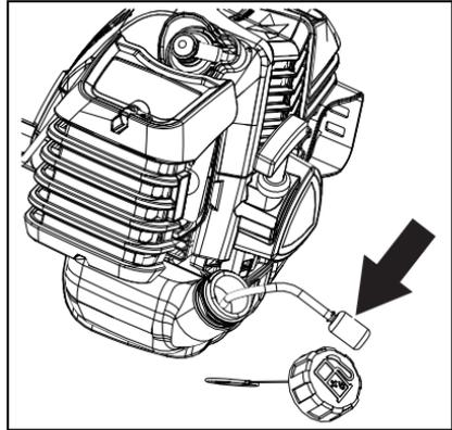
Note: Federal EPA regulations require all model year 2012 and later gasoline powered engines produced for sale in the United States to be equipped with a special low permeation fuel supply hose between the carburetor and fuel tank. When servicing model year 2012 and later equipment, only fuel supply hoses certified by EPA can be used to replace the original equipment supply hose. Fines up to \$37,500 may be enforced for using an un-certified replacement part.
