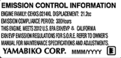
The 50 or 300 hour emission compliance period is the time span selected by the manufacturer certifying the engine emissions output meets applicable emissions regulations, provided that approved maintenance procedures are followed as listed in the Maintenance Section of this manual.
