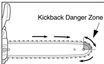
2. Keep a good firm grip on the saw with both hands, the right hand on the rear handle, and the left hand on the front handle, when the engine is running. Use a firm grip with thumbs and fingers encircling the chain saw handles. A firm grip will help you reduce kickback and maintain control of the saw. Don't let go.
