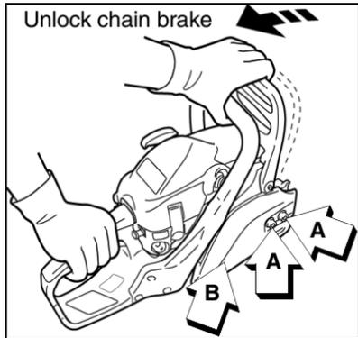
5. Unlock the chain brake, and mount guide bar on studs (C) and slide toward sprocket (E) to make saw chain installation easier. Install chain with cutters on top of guide bar facing forward.
