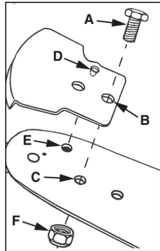
**Guide Bar and Saw Chain Installation/Removal**
