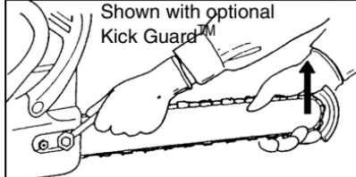
5. Pull the chain around the bar by hand. Loosen the adjustment if you feel tight spots.
