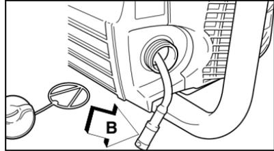
1. Pull Oil Filter out through oil port, and inspect Oil Filter.
