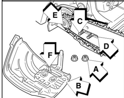
7. Adjust saw chain tension, as instructed in “Adjustment, Chain Tension”.
