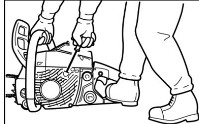
5. Choke may be used if necessary, but after first starting sound, squeeze throttle trigger to release choke and return engine to idle.
