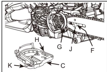
7. Align brake connector (K) on sprocket guard cover (C) to groove on the side of the front hand guard (A). Install and tighten sprocket guard nut (B), finger tight.
