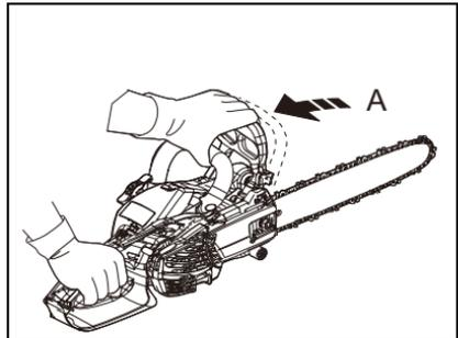
4. The chain starts running when the engine reaches clutch engagement speed (see "Specifications" page).
