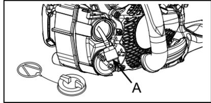
1. Pull filter out through gas port, and inspect filter.
