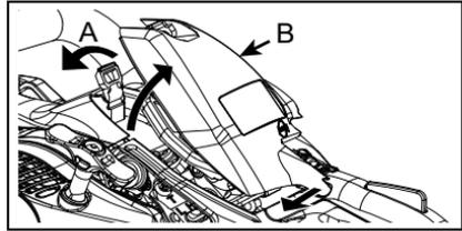
3. Undo the filter cover latch (A), lift the tip of the air filter cover (B), then slide it sideways and remove it.
