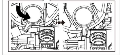
7. Insert the air filter cover (B) into the rear handle side and push it forward, then fix it with the filter cover latch (A).
