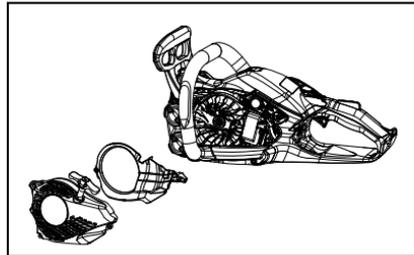
3. Use compressed air or wooden tool to remove dirt and dust from between fins to let cooling air pass easily.
