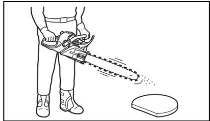
2. Move chain brake lever (A) fully REARWARD to UNLOCK chain brake.
