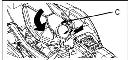
5. Lightly brush dust off air filter, or clean with compressed air, or replace the air filter.
