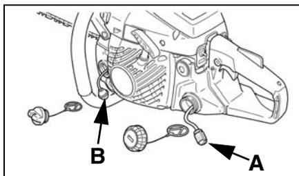
1. Using a wire bent into the shape of a hook, pull filter out through gas port, and inspect filter.
