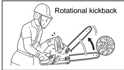
7. Follow instructions in your operator's manual for starting the chain saw and control the chain saw with a firm grip on both handles when it is in operation. Keep handles dry, clean and free of oil. A chain saw should never be carried with the engine running.
