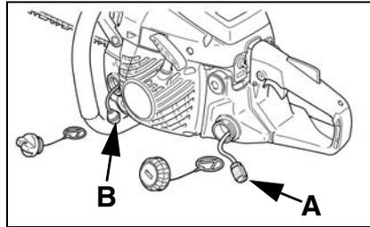
1. Using a wire bent into the shape of a hook, pull filter out through oil port, and inspect filter.
