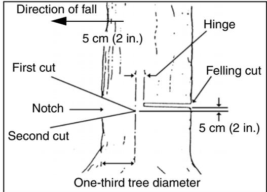
will act as a hinge when the tree falls, guiding it in the desired direction. When the tree starts to fall, kill the engine, place the saw on the ground and make your retreat quickly.
