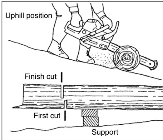
Keep in mind that the wood is heavy and that it will bend and pinch the saw if improperly supported. The trunk will weaken at the point where you make the cut unless the tree is lying on perfectly flat ground or supported as shown. If you make the cut with the tree on the ground, don't let the saw's chain dig into the earth; it is harmful for the saw, and you stand a good chance of being struck by flying debris.
