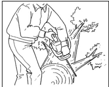
Don't cut with the saw overhead or aligned vertically with your body. If the saw should kickback, you may not have enough control to prevent possible injury.
