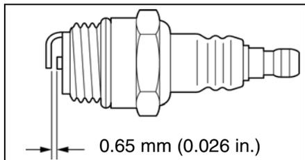
1. Remove air cleaner cover and remove spark plug.
