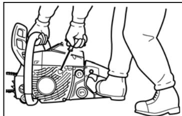
Do not allow recoil handle to snap back against the casing.
