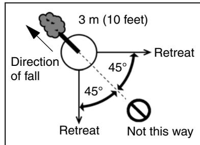
Begin the cut on the side to which the tree is to fall. Cut a notch about 1/3 of the way into the tree. The position of this notch is important since the tree will try to fall "into" the notch. The felling cut is made on the side opposite the notch and at a level about 5 cm (2 in.) above the bottom of the notch. Do not try to cut through to the notch with the felling cut. The remaining wood between the notch cut and felling cut
