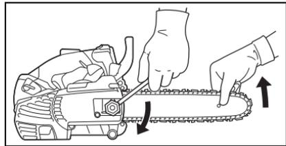
6. Pull the chain around the bar by hand. Loosen the Tension Adjuster if you feel tight spots.
