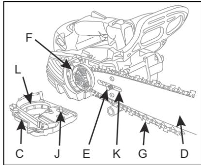
6. Install Saw Chain (G) around Clutch Drum (F) and Guide Bar (D) as shown, with cutters on top of guide bar facing forward.
