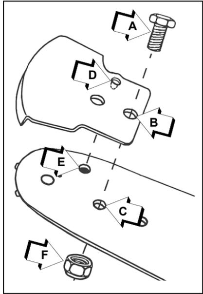
**Guide Bar and Saw Chain Installation / Removal**
