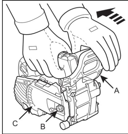
4. Remove Bar/Clutch Cover Nut (B) and remove Bar/Clutch Cover (C).
