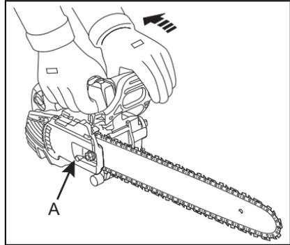
5. Tighten Bar/Clutch Cover Nut with the bar nose held up and under tension.
