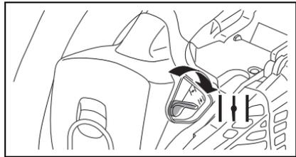
Note: If engine does not start after 5 pulls, use cold start procedure. Do not increase engine speed while chain brake is locked. Severe brake damage will result.
