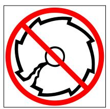
When sharpening a blade, always remove the same amount of materials from each tooth to maintain balance. A blade that is not balanced will cause unsafe handling due to vibration and can result in blade failure.
