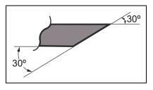
If an electric grinder is used, use care not to overheat teeth, do not allow tips/tooth to glow red or turn blue. DO NOT place blade in cooling water. This will change the temper of the blade and could result in blade failure.
