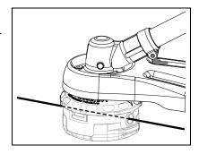
Hold trimmer head while turning 4. knob clockwise to wind line onto spool until about 13 cm (5 in.) of each line remains exposed.
