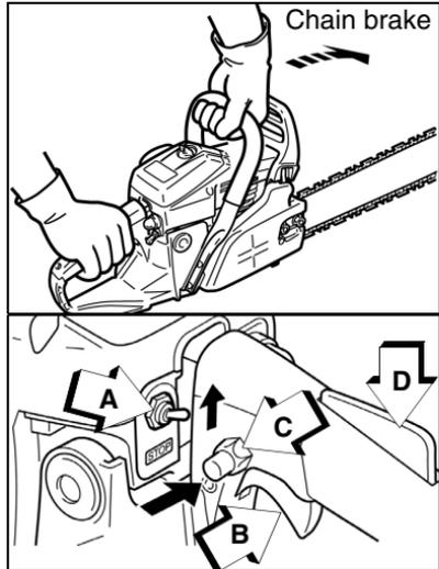
4. Securely hold the chain saw as shown and pull starter handle.
