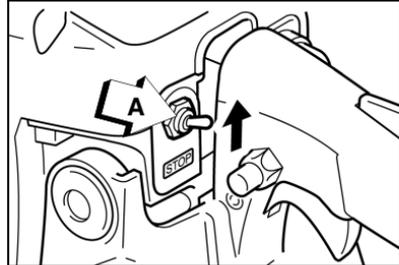
4. Securely hold the chain saw as shown and pull starter handle.
