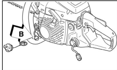
1. Pull filter out through oil port, and inspect filter.
