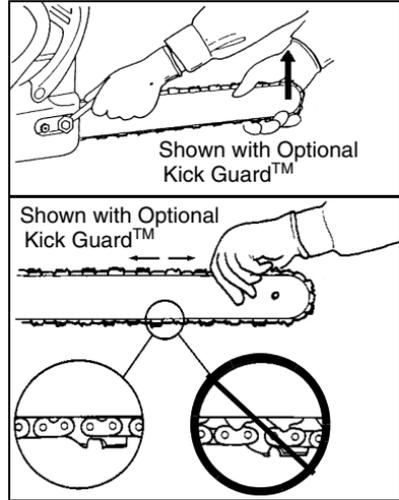
5. Pull the chain around the bar by hand. Loosen the adjustment if you feel tight spots.
