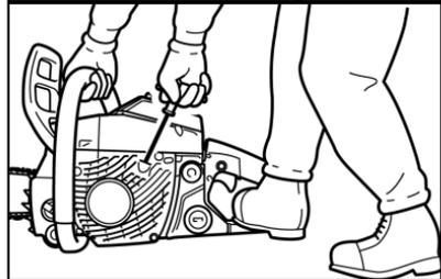
8. Push choke control knob all the way IN (OPEN [↑↓]choke position).
