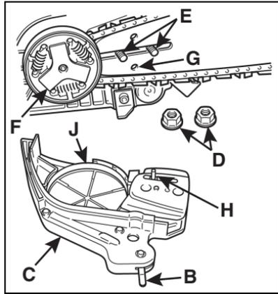
6. Install sprocket guard over guide bar studs. Ensure chain tension adjuster pin (H) fits into the guide bar adjuster hole (G), brake band (J) is positioned around clutch drum (F). Tighten sprocket guard nuts finger tight.
