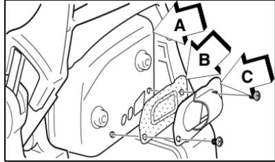
Note: When cleaning carbon deposit, be careful not to damage the catalytic element inside muffler.
