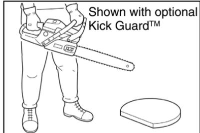
2. Move chain brake lever fully REARWARD to UNLOCK chain brake.
