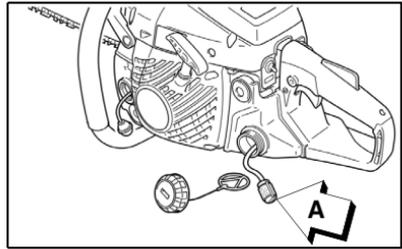
1. Pull filter out through gas port, and inspect filter.
