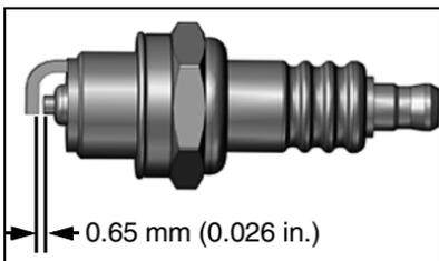
1. Remove air cleaner cover and remove spark plug.
