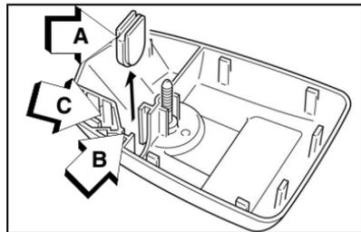
Note: For operation at normal temperature (5°C [41°F]) return the plug to its original position. To prevent over-heating of the engine.
