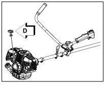
fully depress throttle trigger to wide open position. Rapidly pull recoil starter handle/rope (D) until engine fires (or maximum five pulls).
