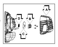
Note: When cleaning carbon deposit, be careful not to damage the catalytic element inside muffler.
