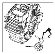
6. When the inside of the fuel tank is dirty, rinse the tank out with gasoline to clean it.
