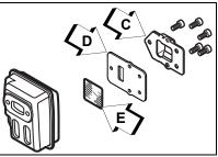
3. Use a wood or plastic scraping tool to clean deposits from cylinder exhaust port (C).
