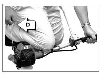
move choke lever back to RUN ( $|\downarrow\downarrow|$ ) position. Firmly grasp throttle handle and throttle trigger lockout with left hand and fully depress throttle trigger to wide open position. Pull recoil starter handle/rope until engine starts and runs. Release throttle trigger, and allow unit to warm up at idle for several minutes.
