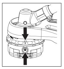
Insert one end of trimmer line into an eyelet, and push line equal distance through trimmer head.
