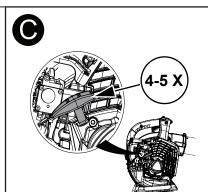
Note: If after 5 pulls the engine does not start, perform Cold Start procedure.
