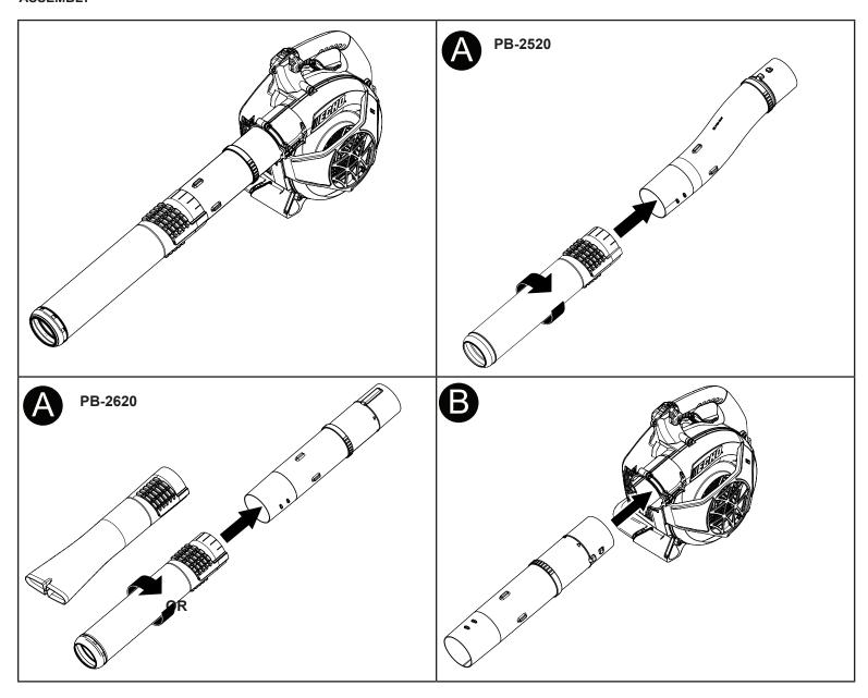
Note: Align tabs on tube with slot on unit. Insert until "CLICK" is heard.
