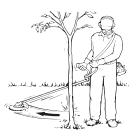
To free a blade that is bound in the cut, stop the engine, and support the trimmer or brushcutter to keep stress off the blade. Push the tree away from the entry point of the cut to open the cut, and pull the blade directly away from the cut in a straight-line motion. Use caution when releasing the tree to avoid being struck by spring-back or falling.
