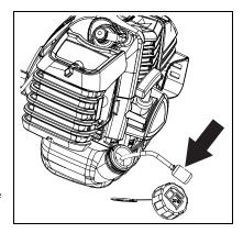
When the inside of the fuel tank is dirty, rinse the tank out with gasoline to clean it.
