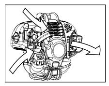
Removal of cooling passage blockages or cleaning of cooling fins is considered "Normal Maintenance." Any failure attributed to lack of maintenance is not warranted.
