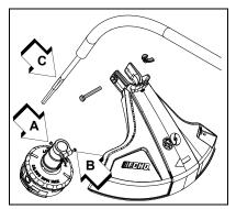
5. Install the bearing housing and shield.
