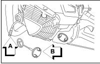
6. Push the Oil Filter (A) into the tank, service with oil and install the Oil Cap (B).
