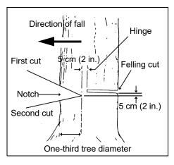
direction. When the tree starts to fall, kill the engine, place the saw on the ground and make your retreat quickly.
