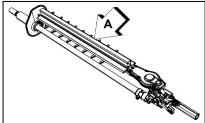
2. Hold blade adjustment handle (B) and compress blade lock levers (C) and (D) together. Rotate blade to desired position. Release levers to lock blade.
