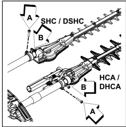
2. Pull the drive shaft (C) from the housing, wipe clean, then apply 15 ml (0.5 oz.) of grease.
