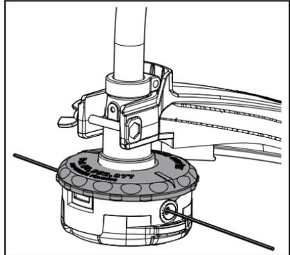
4. Hold trimmer head while turning knob clockwise to wind line onto spool until about 13 cm (5 in.) of each line remains exposed.
