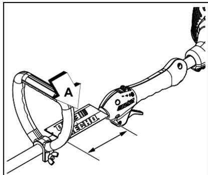
1. Position Support Handle (A) in comfortable operating position and tighten wing nut (B). The cutting attachment should be 5 - 7.5 cm (2 - 3 in.) above the ground and as level as possible.
